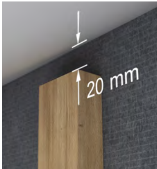
The battens should be positioned 10 mm higher than the recommended clearance and 20 mm down from the soffit/window cill to accommodate the 10mm drip edge to the weatherboard.
