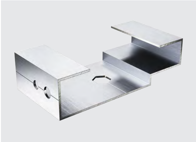
Hanger Type C Hanger with pre-applied drilling, usually with internal thread, for fine adjustment of the facade panel and additional hole for setting a locking screw. A fixed point is created when the locking screw is set. As an alternative to the locking screw, side-mounted locking brackets can also be used.
