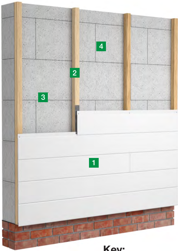
Typical horizontal Hardie® VL Plank installation
