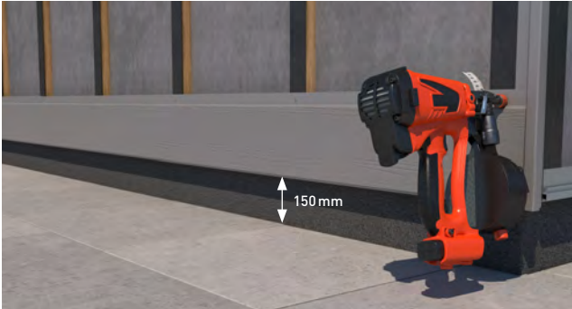
Hardie® VL Plank should be installed 150 mm above soft terrain.
